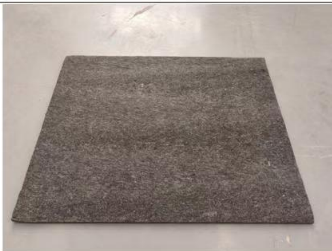
20mm Thick PET Sound-absorbing Material with a Surface Density of 1.44kg (Only Used for Installation of Samples)
